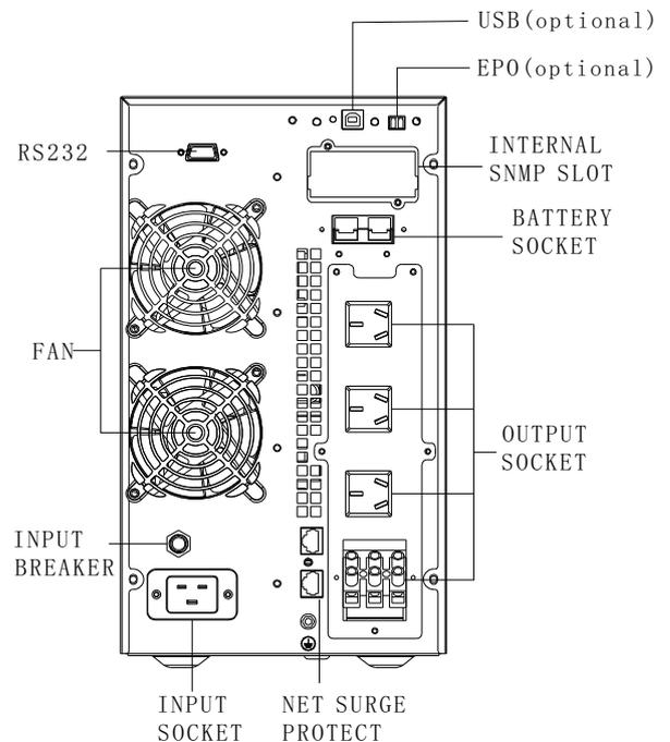
Fig. 2 2/3KVA Rear Panel view
