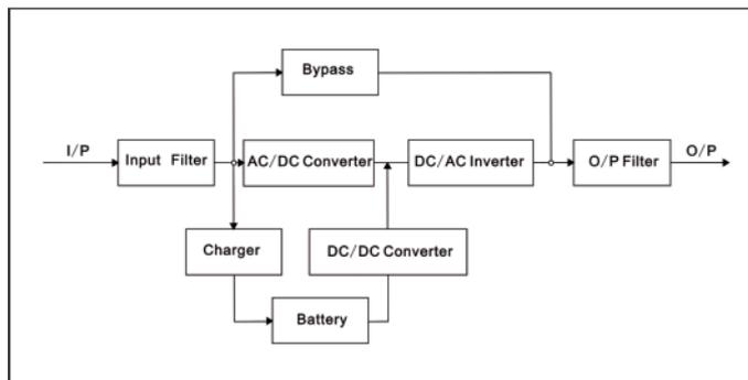
Fig 4 UPS Principle Diagram
