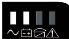
When the mains power down or instable, UPS will turn to battery mode at once.
