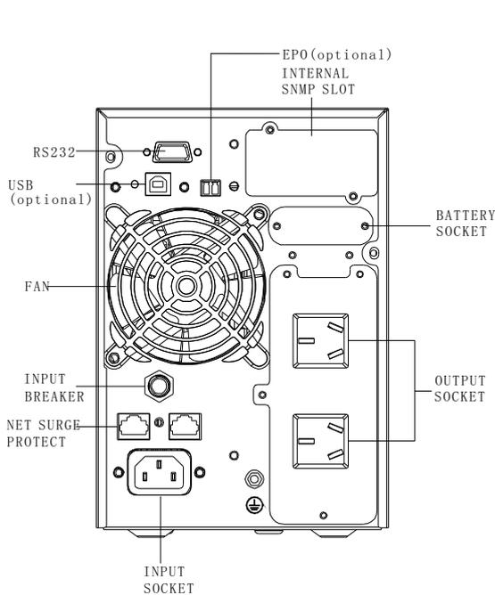
Fig. 1 1KVA Rear Panel view
