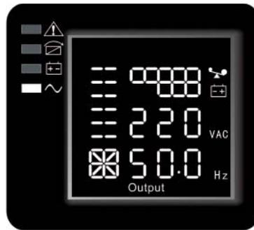
Fan-status graphics section—display if the fan works normally. When the fan works normally, it will show the dynamic fan blades rotating; when the fan works abnormally, the icon \* will keep on flashing with the warning .
